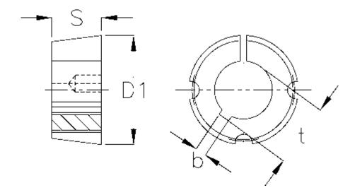
$\begin{array}{lll} b & = 10 \\ Bore & = 38 \\ Bush type & = 2012 \\ D1 & = 70 \\ S & = 31,8 \\ Screw size & = 7/16 \times 7/8" \\ t & = 41.3 \\ Transmission moment = 808 \end{array}$
